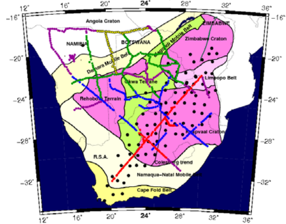
Figure 2: SAMTEX MT station locations. Phase I - red; Phase II - blue; Phase III - green; Phase IV - purple; DeBeers – yellow; SASE sites - black. The interpreted tectonic subdivision is from S. Webb (unpubl.).
