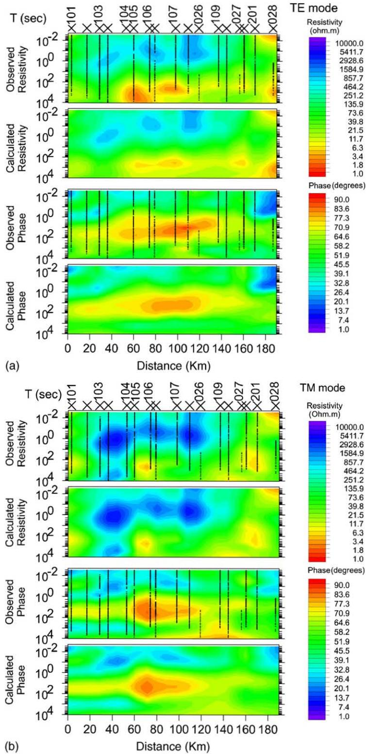
Fig. 2. (a) Pseudosections of TE mode apparent resistivity and phase of the observed and the modelled data with data points shown on observed data contours. (b) Pseudosections of TM mode apparent resistivity and phase of the observed and the modelled data with data points shown on observed data contours.
