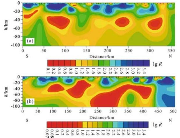
Fig. 3 Line 500 (a) and line 600 (b) resistivity models from 2D MT inversion
