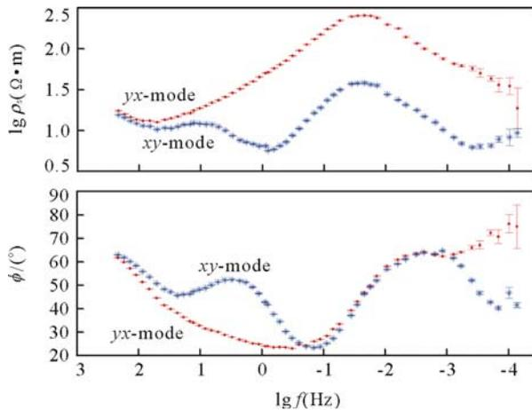
Fig. 2 Super-wide band MT sounding curve of site Tbt-628
