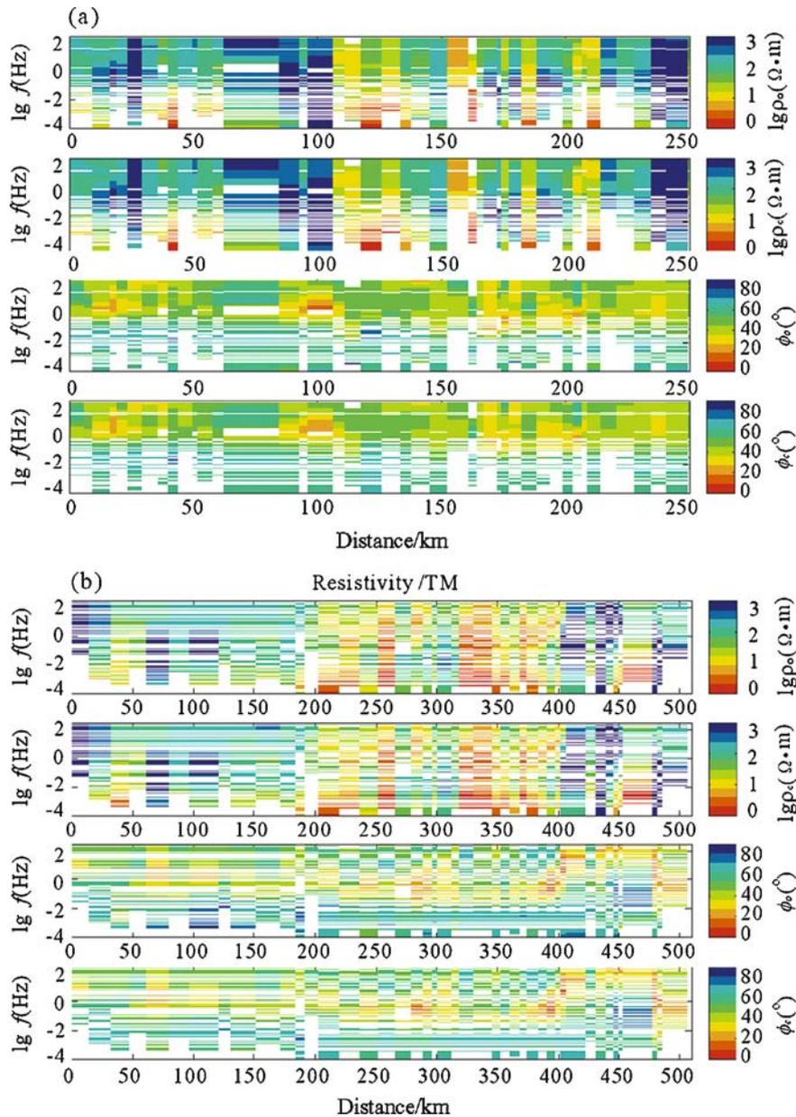
**Fig. 4** Observed and calculated MT pseudo-sections of line 500 (a) and line 600 (b)
