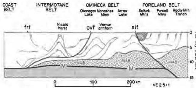
Fig. 2 Cartoon of the seismic interpretation from Cook et al. (1992). NAB: North American Basement; M: Moho; frf: Fraser River fault; ovf: Okanagan Valley fault; slf: Slocan Lake fault.
