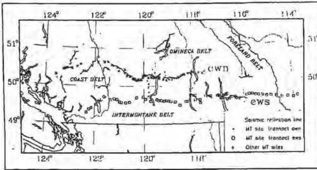
Fig. 1 Locations at which seismic and MT measurements were made in southern British Columbia. MT date interpreted in this paper came from the two east-west transects labeled *ews* and *ewn*. Kootenay Lake lies directly below the label *ewn*.
