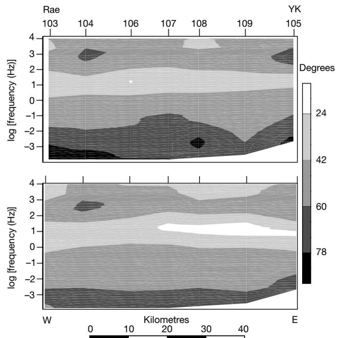
**Figure 2** Contoured magnetotelluric phase responses for the seven sites from Yellowknife to the surface expression of the western boundary of the Slave craton. Distance is along the abscissa, and log(frequency) is along the ordinate. Top, phases with the electric component directed N41W. Bottom, phases with the electric component directed N49E.
