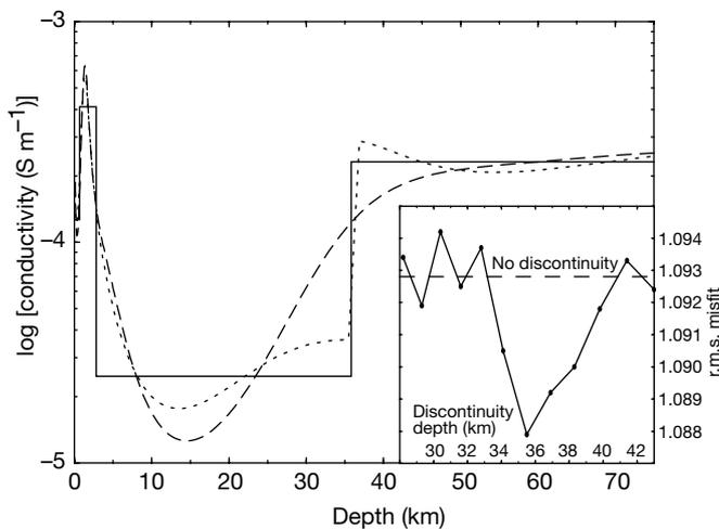
**Figure 4** One-dimensional conductivity–depth models that fit the averaged impedances<sup>21</sup> of the responses shown in Fig. 3. Solid line, best-fitting layered-Earth model. Dashed line, best-fitting continuous model. Dotted line, best-fitting continuous model with a permitted step change at 35.5 km. Inset, r.m.s. misfit for best-fitting continuous models varying the depth to the permitted step change.
