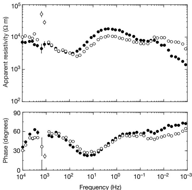
**Figure 3** Magnetotelluric response from a central site on the profile, site 106 (Fig. 2). Filled circles, responses with the electric component directed N41W; open symbols, responses with the electric field directed N49E.
