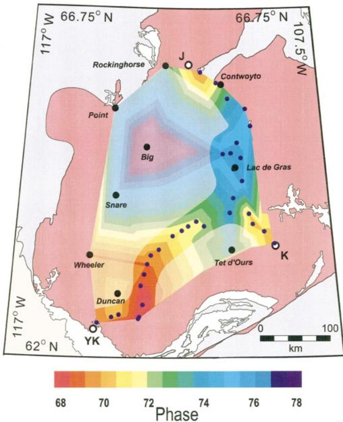
**Figure 2.** Map of averaged magnetotelluric phases at 300 s period based on data from land sites (small dots) and preliminary processing of 1998–1999 lake-bottom sites (large named dots). YK—Yellowknife; J—Jericho pipe; K—Kennady lake pipes. On Slave craton at 300 s period, electromagnetic waves are penetrating 100–150 km into lithosphere. VE—vertical exaggeration.
