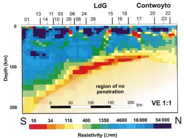
**Figure 3.** Resistivity model of winter road magnetotelluric data projected along north-south profile A-B (Figure 1). LdG—Lac de Gras.
