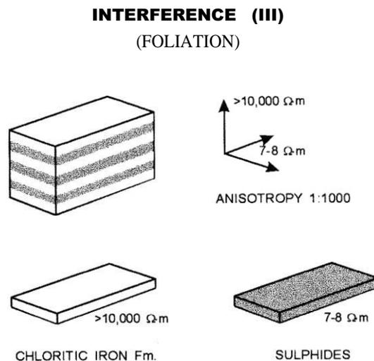
Figure 1: One of the anisotropic mechanisms (Katsube et al, 1996b). The chloritized iron formation sample consists of inter-layered sulphide-rich material (7 to 8  $\Omega\text{-m}$ ) and non-sulphide material (greater than 10,000  $\Omega\text{-m}$ ), resulting in electrical resistivities of 7 to 8  $\Omega\text{-m}$  in directions parallel to the foliation, and of greater than 10,000  $\Omega\text{-m}$  in the directions perpendicular to the foliation.
