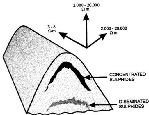
*Figure 4: A folded gneissic rock sample with sulphide layers accumulated near the head of the fold, forming a zone of high electrical conductivity along its axis (Katsube et al., 1996c).*
