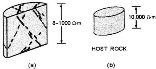
Figure 2: Another anisotropic mechanism (Katsube et al., 1996b). Thin veins (less than 1 mm thick) containing sulphides cut across metamorphosed foot wall sediment material, reducing the electrical resistivity of the bulk rock from over 10,000  $\Omega\text{-m}$  (estimated) to 8 to 1,000  $\Omega\text{-m}$ , in the direction of the vein.
