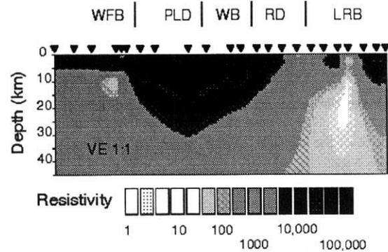
Figure 5: Preliminary resistivity model for the MT data along the 1994 profile. The inverted triangles show the locations of the sites. Grey scale as Fig. 4.
