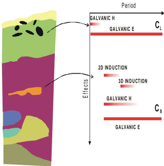
**Figure 3.** Cartoon of the different inductive and galvanic effects that appear in a MT mining scale survey.
